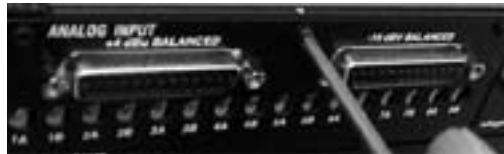
Attaching the card faceplate into the back panel surface of the 192 I/O
