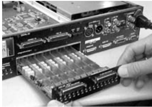
Lifting slightly while pushing the card back into the bay
